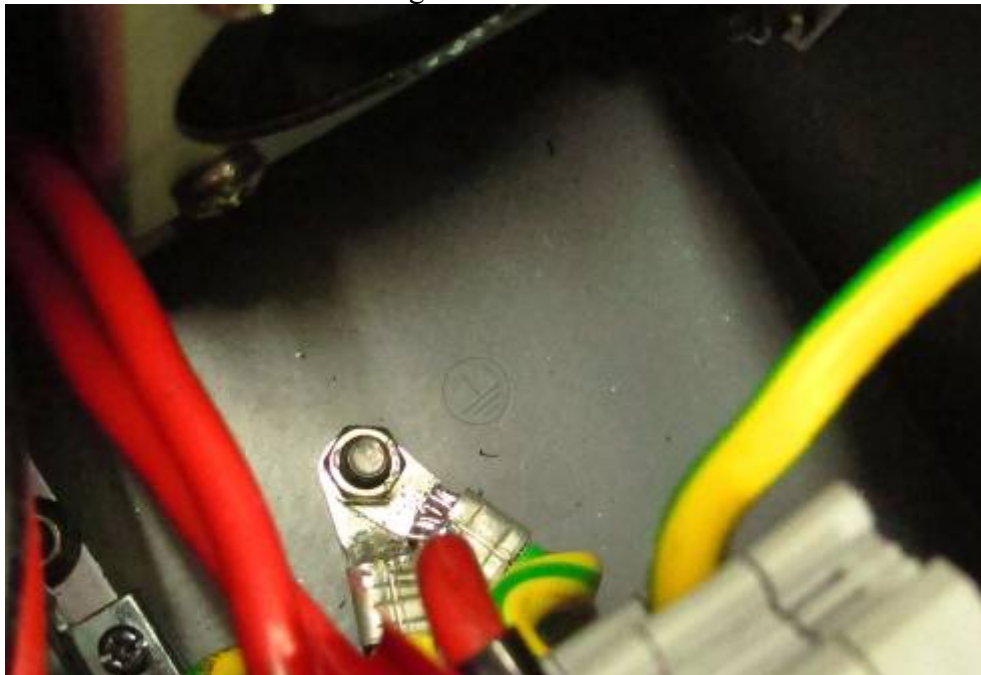
Earthing terminal of the unit
