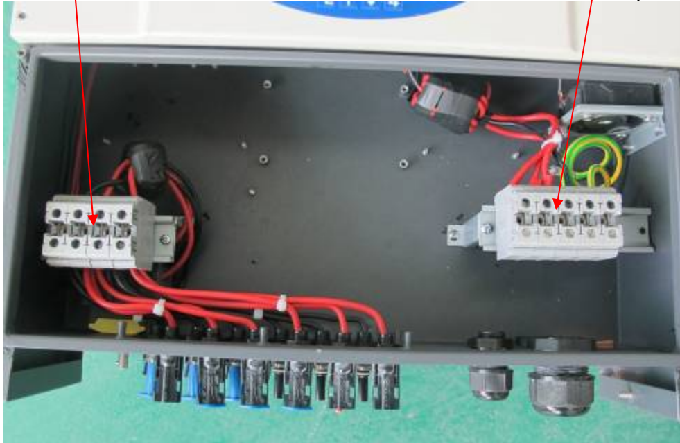
Earthing terminal of the unit
